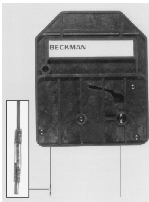
Fig. 1. SPE device installed on the inlet capillary of a Beckman P/ACE capillary cartridge. A magnified view of the device is presented inset and shows the polypropylene extractor tube containing Rezorian material and plugged at both ends by capillaries.
